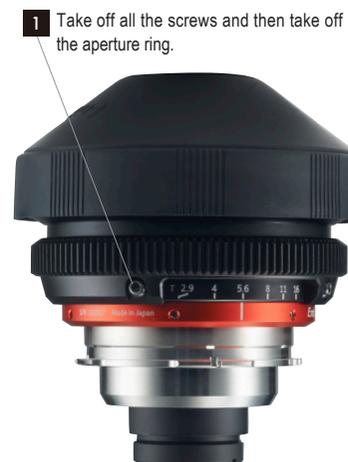
When disassembling the lens, please make sure that the front lens faces up. The parts might fall and damage the lens.
